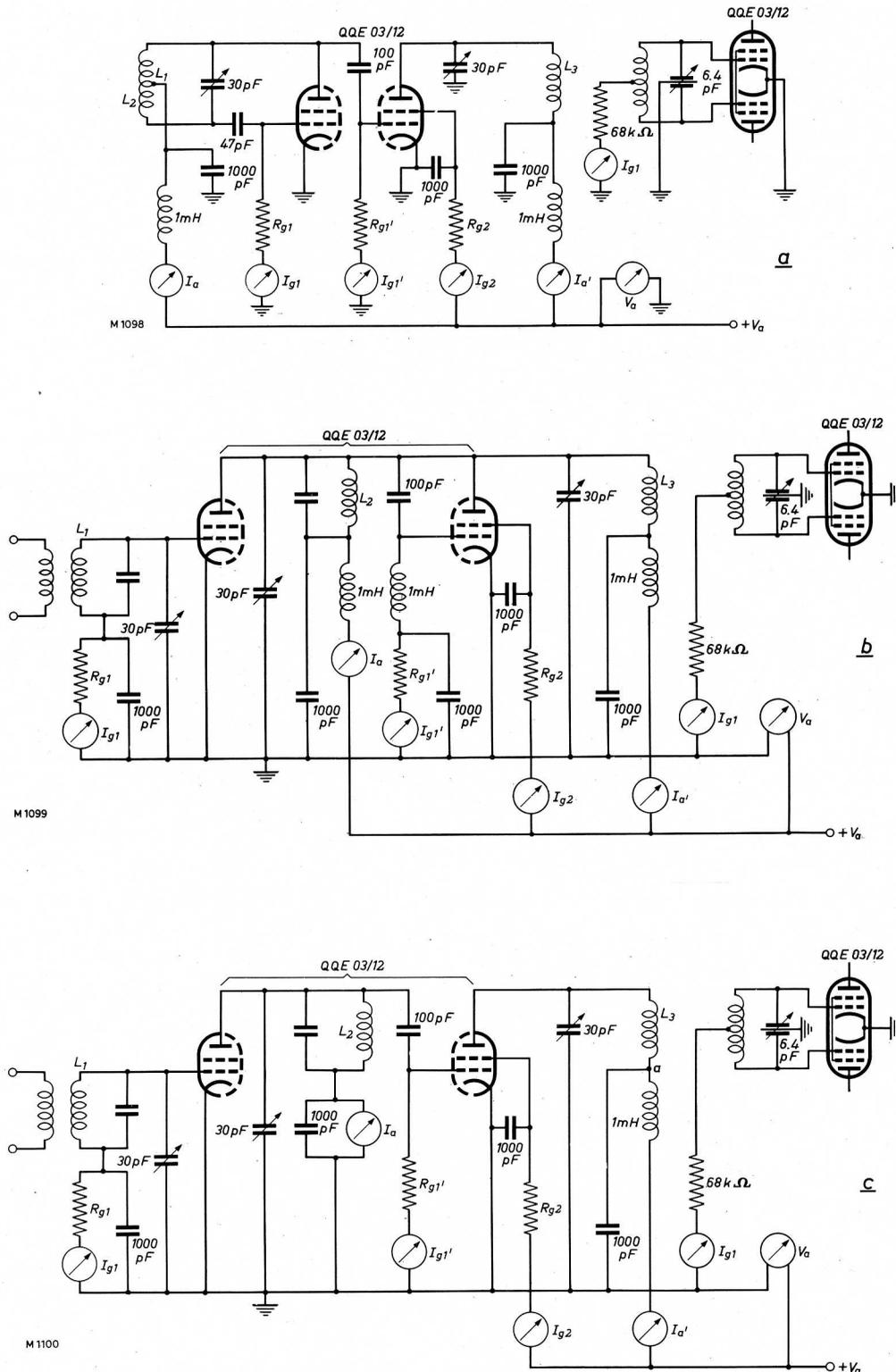
Fig. 24. Circuits of two-stage multipliers with one QQE 03/12.
