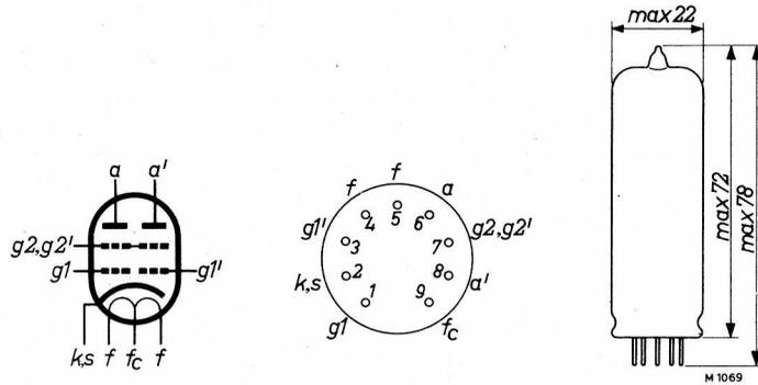
Fig.3. Socket connections and dimensional drawing (dimensions in mm) of QQE 03/12.
