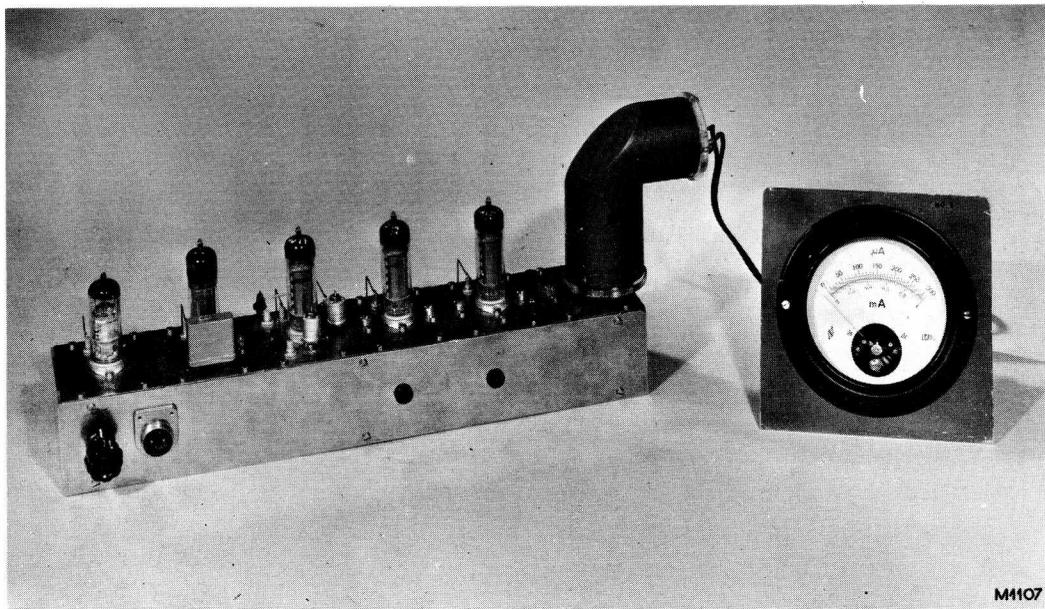
Fig.30. 200 Mc/s transmitter with modified modulator stage.
