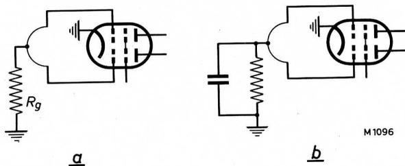
Fig.22. The best symmetry is obtained when a single grid-leak is used, bypassed to earth; (a) incorrect, (b) correct.
