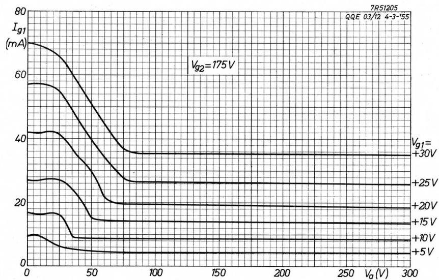
Fig. 8, 9 and 10. Anode current  $I_a$ , screen grid current  $I_{g2}$  and control grid current  $I_{g1}$  as functions of the anode voltage  $V_a$  with the control grid voltage  $V_{g1}$  as parameter at a screen-grid voltage  $V_{g2} = 175V$  (all current values per unit).
