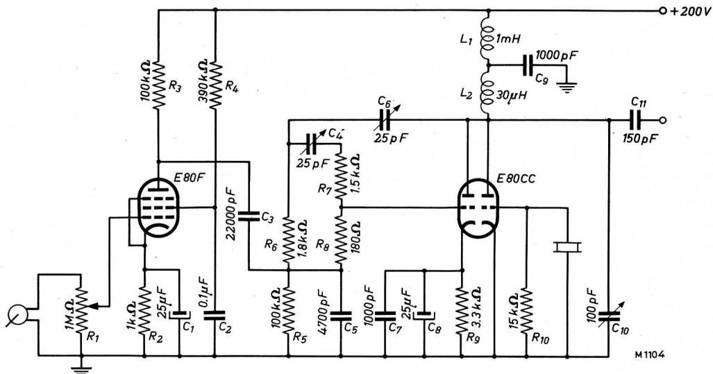
Fig.28. Modified modulator stage of the 200 Mc/s transmitter.
