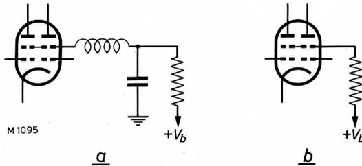
Fig.21. The screen-grid resistor should not be bypassed, and no choke be used in the screen-grid lead; (a) incorrect, (b) correct.
