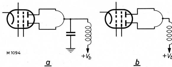
Fig.20. Connecting the H.T. supply to the anode circuit; (a) incorrect, (b) correct.
