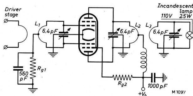
Fig.23. Push-pull output stage with QQE 03/12.
