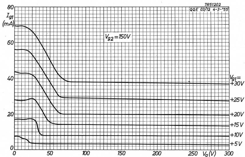
Fig. 5. 6 and 7. Anode current  $I_a$ , screen grid current  $I_{g2}$  and control grid current  $I_{g1}$  as functions of the anode voltage  $V_a$  with the control grid voltage  $V_{g1}$  as parameter at a screen-grid voltage  $V_{g2} = 150 V$  (all current values per unit).
