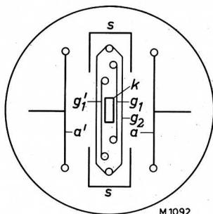
Fig. 2. Cross-sectional drawing of the QQE 03/12.
