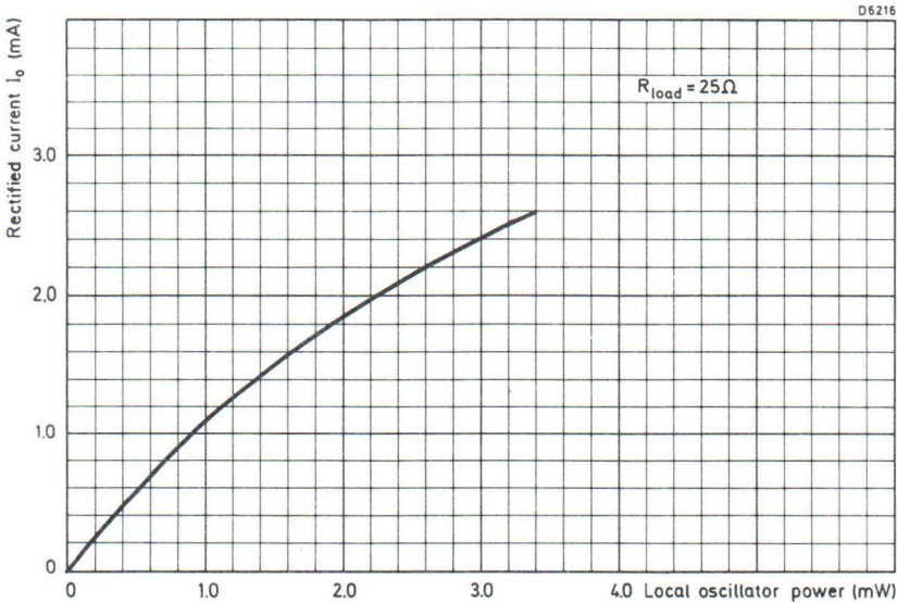
Fig.2 Typical rectified current as a function of local oscillator power at 34.86 GHz
