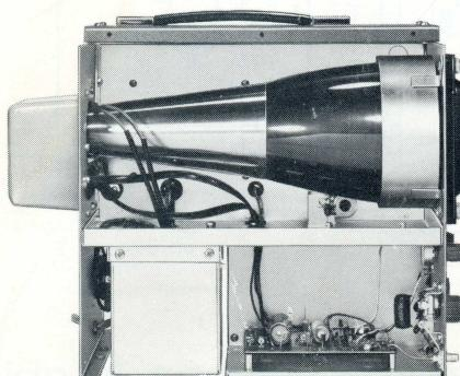
izontal input allows the sweep signal to be applied by an external generator. The front panel internal-external switch and external sync connector provide a means for applying an external sync signal. A one volt peak-to-peak output provides a signal that can be used as a comparison to determine the value of an unknown voltage.
