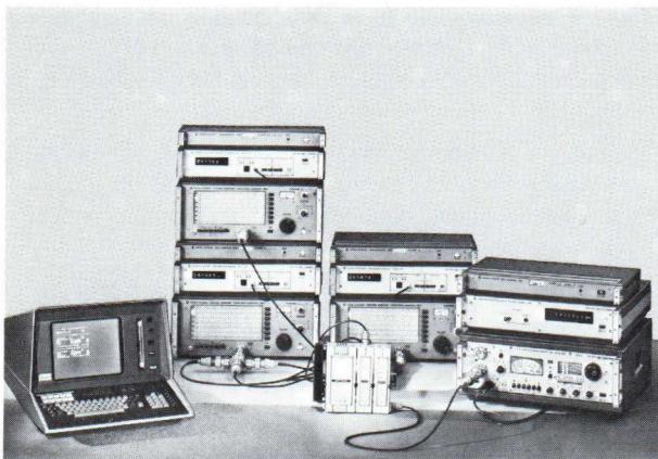
Automatic test assembly for intermodulation and crossmodulation measurement (3x SMLU plus SMLU-Z and PCW, ESU 2 plus EZK and PCW, Tektronix desktop calculator 4051)
