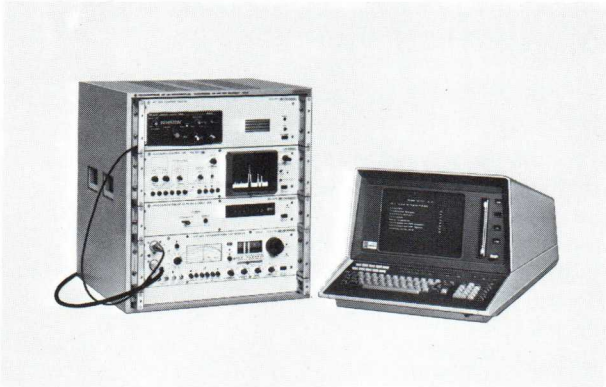
Automatic VHF-UHF test assembly for wanted- and unwanted-signal measurements (MSUP plus Tektronix desktop calculator 4051)
