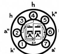
The BRIMAR 6058 is a trustworthy miniature double diode designed for reliable operation under severe conditions of vibration and shock.
