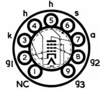
The BRIMAR type 6059 has been specially designed for use in the early stages of high gain A.F. amplifiers. Its thorough screening and rigid construction ensure low microphony and greatly reduced hum.
