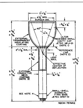
NOTE : THE PLANE THROUGH THE TUBE AXIS AND VACANT PIN POSITION 3 MAY VARY FROM THE PLANE THROUGH THE TUBE AXIS AND ULTOR TERMINAL BY AN ANGULAR TOLERANCE (MEASURED ABOUT THE TUBE AXIS) OF  $\pm$  100. THE ULTOR TERMINAL IS ON SAME SIDE AS VACANT PIN POSITION 3.
