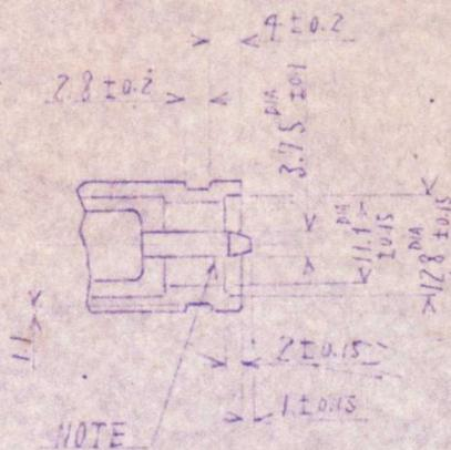
Note: Output Inner Conductor to be Concentric with Inside Dia of Outer Conductor within 0.013mm.
