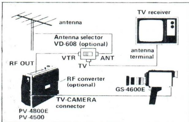
NOTE: When you only monitor the recorded tape on the TV receiver, you do not need to connect the camera to the VTR. Just set the TV-CAMERA switch to TV, and playback monitoring is possible using the VTR function lever.
