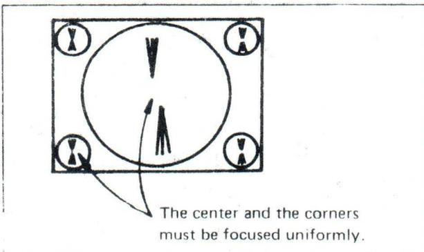
(2) Adjustment of scanning size and the centering
