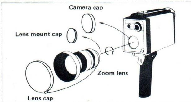
NOTE: The ring at the end of the zoom lens is to hold the lens cap. When mounting the zoom lens, do not remove this ring.
