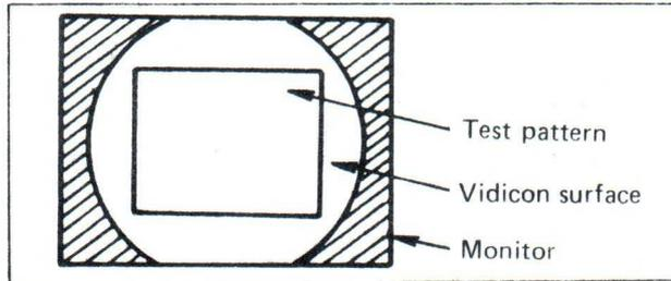
Zoom the camera lens until the resolution pattern as large as possible so that the pattern is not distorted. Keeping the camera and lens in this condition, adjust R69 (H. size) and R95 (V. Height) again for a correct aspect ratio. i.e.: The wedges at top and bottom of the test pattern, also the wedges on the sides of the test pattern reach the vertical and horizontal raster limits.
