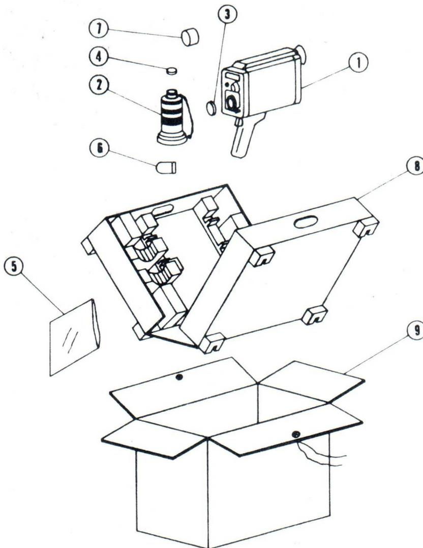
1. Remove the zoom lens ② from the camera ①, and attach the vidicon cap ③ to the lens mount of camera.
