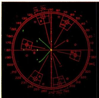
Fig. VII-19. Vectorscope display of the "PHASE"-pattern
