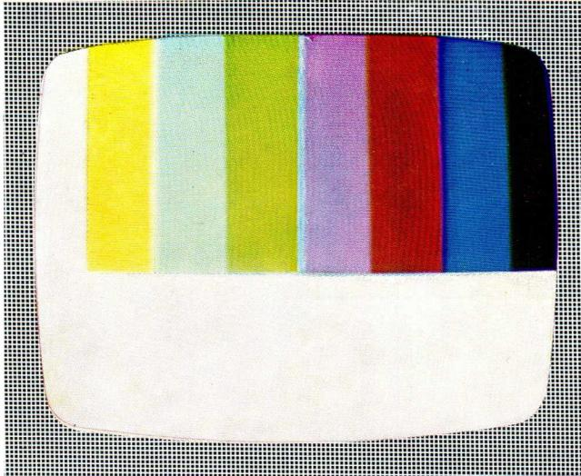
Fig. VII-25. "COLOUR BAR"-pattern
