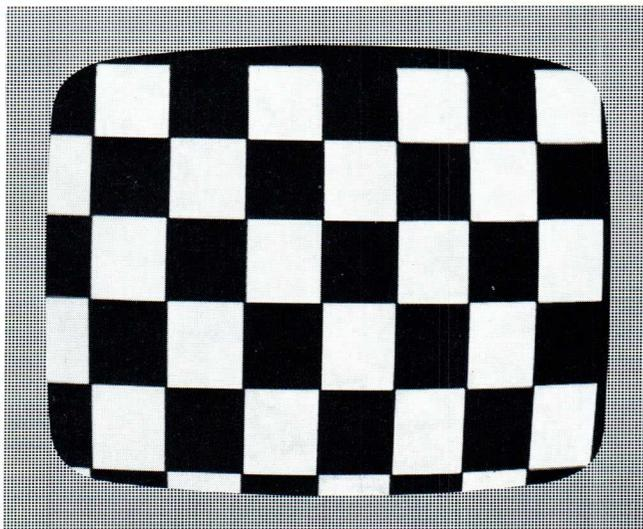
Fig. VII-3. Incorrect centring
