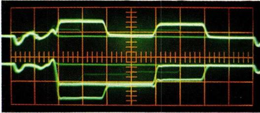
Fig. VII-35. Only (B-Y) demodulator adjusted incorrectly
