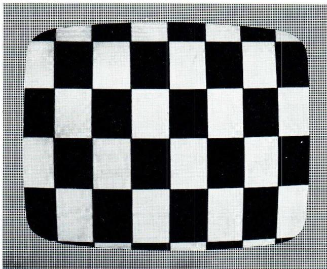
Fig. VII-2. Incorrect vertical amplitude and linearity
