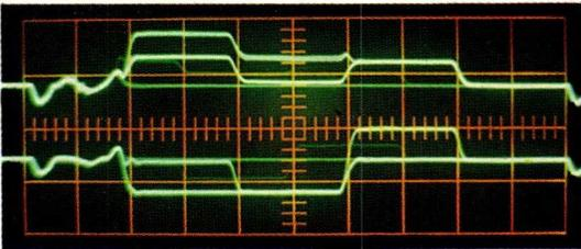
Fig. VII-36. Both demodulators adjusted incorrectly
