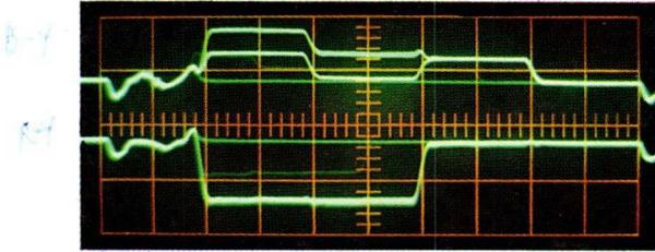
Fig. VII-34. Only (R-Y) demodulator adjusted incorrectly
