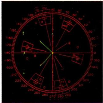
Fig. VII-24. Vectorscope display of the "MATRIX"-pattern
