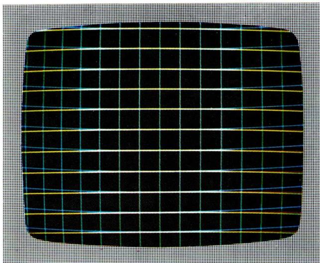
Fig. VII-11. Incorrect horizontal dynamic convergence
