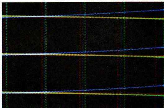
Fig. VII-12. Picture detail in case of incorrect dynamic convergence
