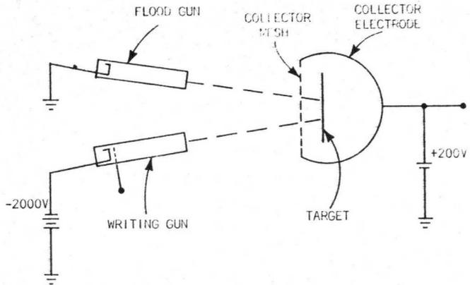
Fig. 3-4. Floating target control with two guns.
