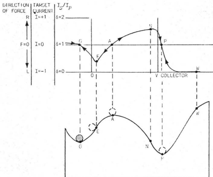
Fig. 3-3. Mechanical stability model and secondary-emission curve.
