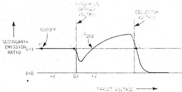
Fig. 7-6. Secondary-emission curve.
