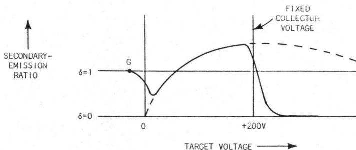
Fig. 2-5. Secondary-emission curve modified by fixed collector voltage.
