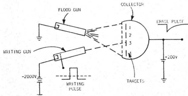
Fig. 4-1. Control of multiple targets with two guns.
