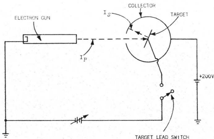
Fig. 3-1. Secondary-emission circuit modified to allow floating target.
