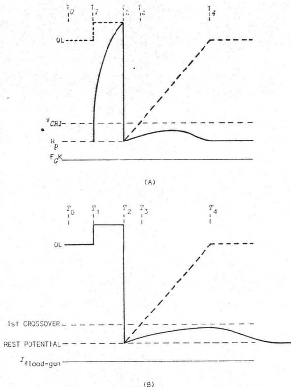
Fig. 6-17. Composite target element erasure.
