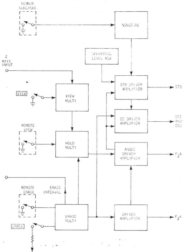
Fig. 8-23. Data-display storage block diagram.
