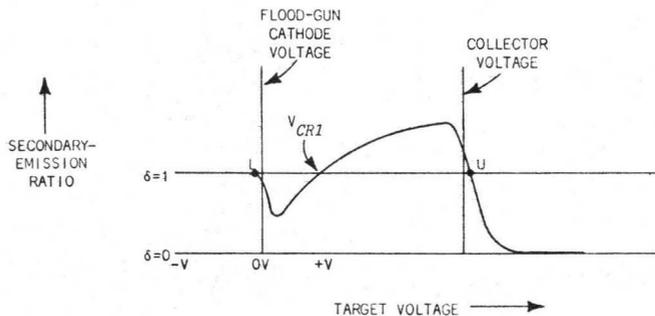
Fig. 7-4. Secondary-emission curve.
