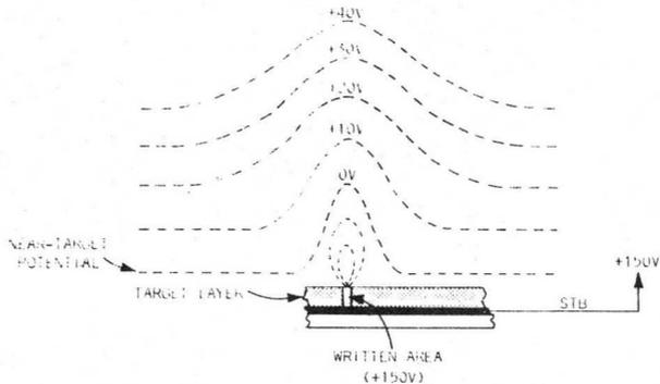
Fig. 6-8. Near-target potential distorted by written charge.
