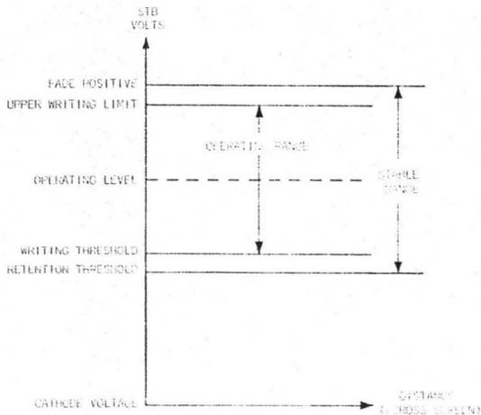
Fig. 5-4. Storage-target-backplate voltage versus distance across screen.
