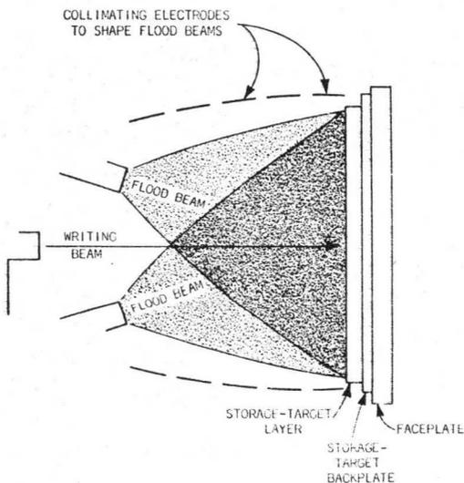
Fig. 6-1. Collimation system.
