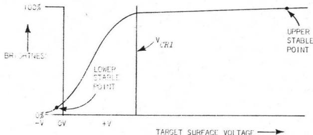
Fig. 7-5. Bistable brightness curve.
