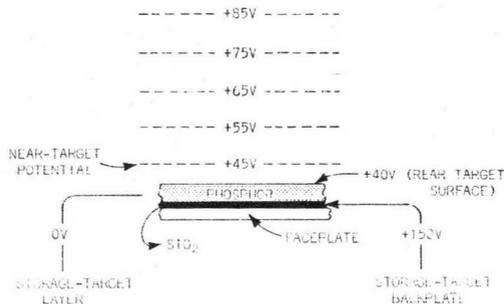
Fig. 6-7. Near target potential line.
