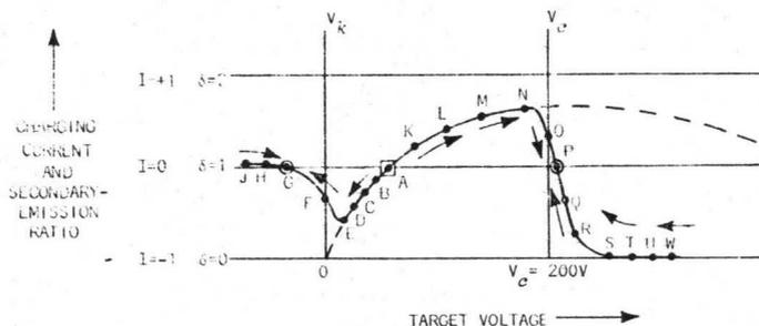
Fig. 3-2. Secondary-emission curve - fixed collector voltage.
