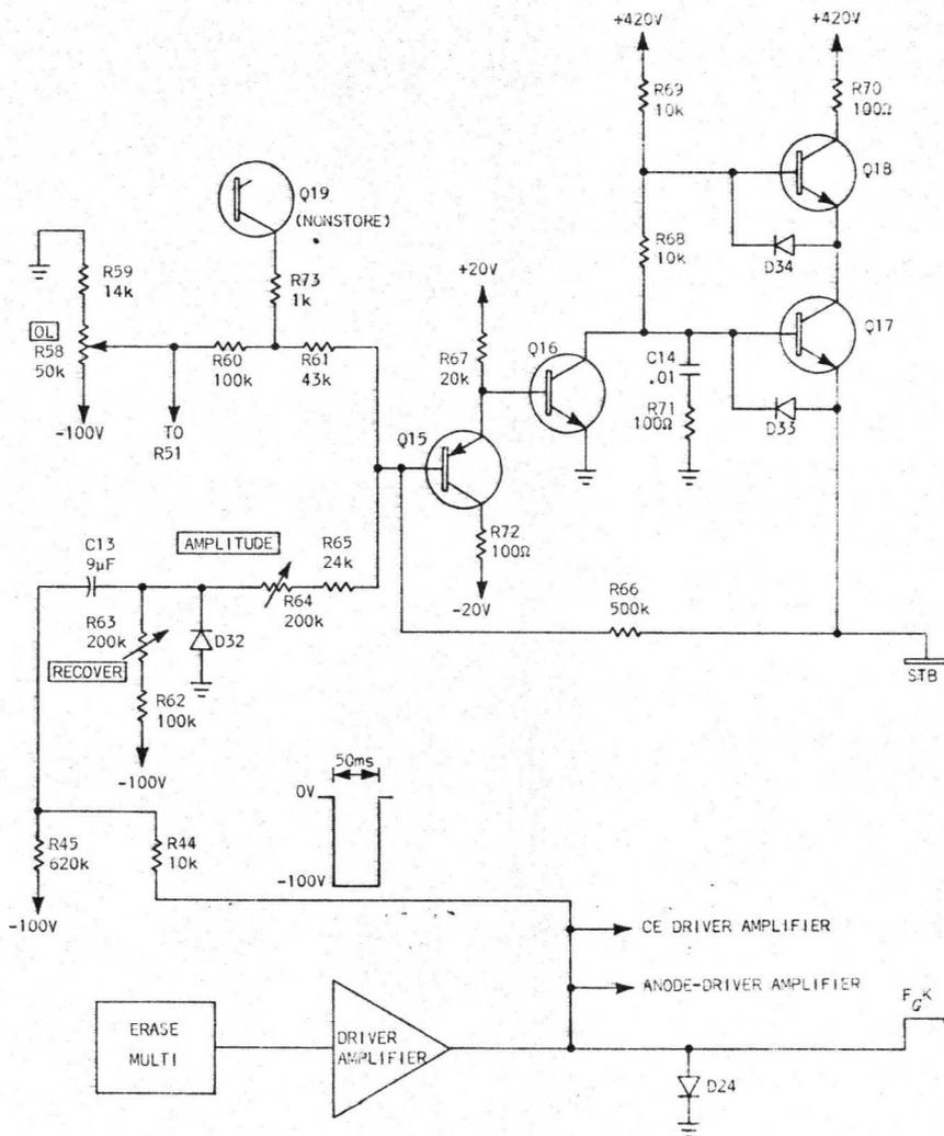
Fig. 8-34. SIB driver amplifier schematic.
