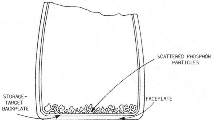
Fig. 5-2. Scattered-particle tube.
