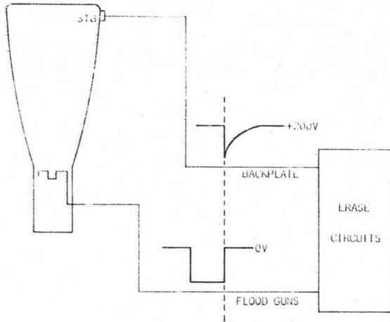
Fig. 6-18. Both flood gun and backplate erase pulsed.
