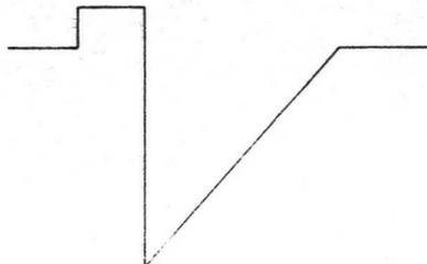
Fig. 6-13. Backplate erase pulse.
