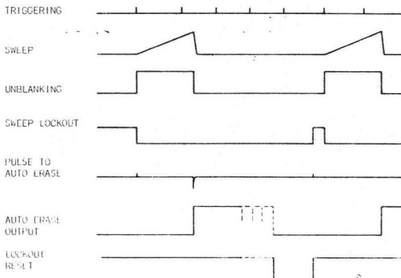
Fig. 8-12. Oscilloscope waveforms when using auto erase.
