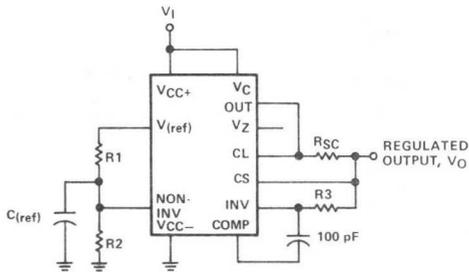
NOTES: A.  $R_3 = \frac{R_1 \cdot R_2}{R_1 + R_2}$  for minimum  $\alpha V_O$ .
