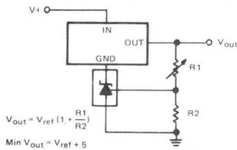
FIGURE 11—OUTPUT CONTROL OF A THREE-TERMINAL FIXED REGULATOR
