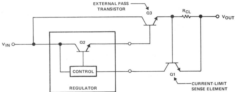
Figure 4.6. Constant-Current Limiting for External Pass Transistor Applications
