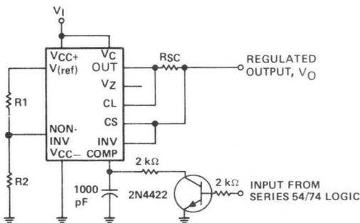
NOTE A: Current limit transistor may be used for shutdown if current limiting is not required.
