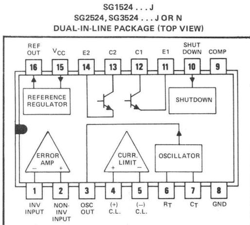
The SG1524 is characterized for operation over the full military temperature range of  $-55^{\circ}\text{C}$  to  $125^{\circ}\text{C}$ . The SG2524 and SG3524 are characterized for operation from  $0^{\circ}\text{C}$  to  $70^{\circ}\text{C}$ .
