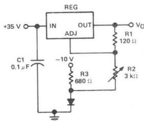
FIGURE 2—0-V to 30-V REGULATOR CIRCUIT
