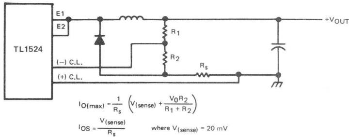
FIGURE 7—FOLDBACK CURRENT LIMITING FOR SHORTED OUTPUT CONDITIONS
