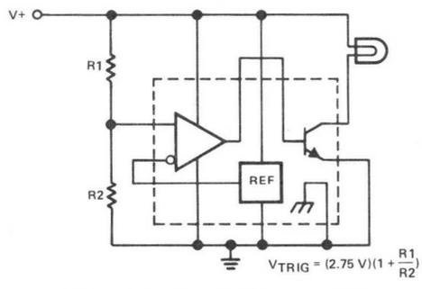
FIGURE 4—OVER-VOLTAGE DETECTOR
