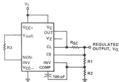
NOTES: A.  $R_3 = \frac{R_1 \cdot R_2}{R_1 + R_2}$  for minimum  $\alpha V_O$ .
