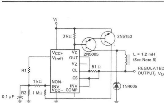
FIGURE 9—POSITIVE SWITCHING REGULATOR
