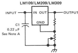
NOTE A: C1 is required if regulator is not located in close proximity to power supply filter.
