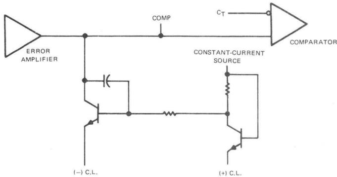
FIGURE 8—CURRENT-LIMIT SCHEMATIC
