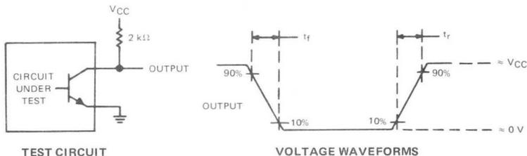
FIGURE 2—SWITCHING TIMES
