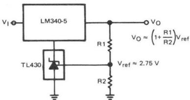
FIGURE 6—ADJUSTABLE SUPPLY WITH STABLE OUTPUT FROM 8 VOLTS TO 35 VOLTS
