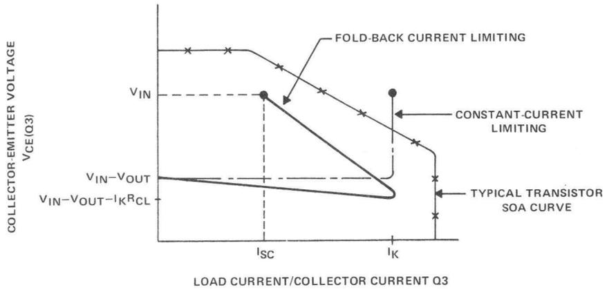
Figure 4.10. Fold-Back Current Limit Safe Operating Area
