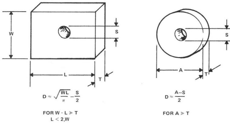
Figure 5.8. Determining "D" for Use with Figure 5.10
