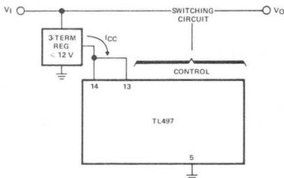
EXTENDED INPUT CONFIGURATION WITHOUT CURRENT LIMIT
