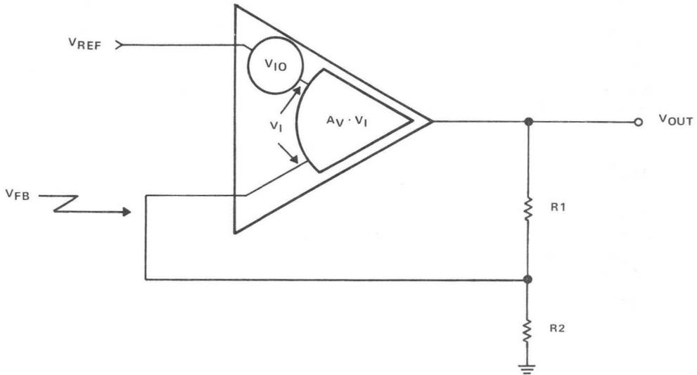
Figure 2.6. Comparator Model Showing Input Offset Voltage Effect
