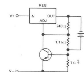
‡ This resistor sets peak current (0.6 A for 1 Ω).
