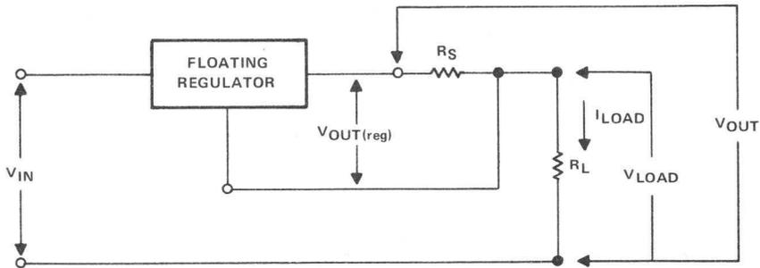
Figure 3.7. Floating Regulator as a Constant-Current Regulator
