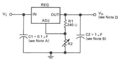
FIGURE 1—ADJUSTABLE VOLTAGE REGULATOR
