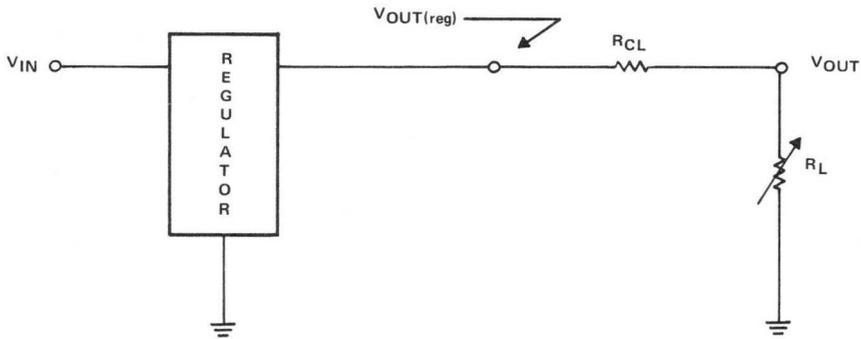
Figure 4.3. Series Resistance Current Limiter
