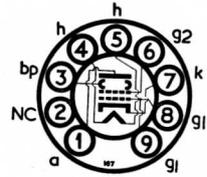
The BRIMAR type 6062, owing to its small size and comparatively high ratings, is very suitable for use in portable V.H.F. equipment. Sufficient ventilation must be provided to ensure that the bulb temperature never exceeds 250°C.
