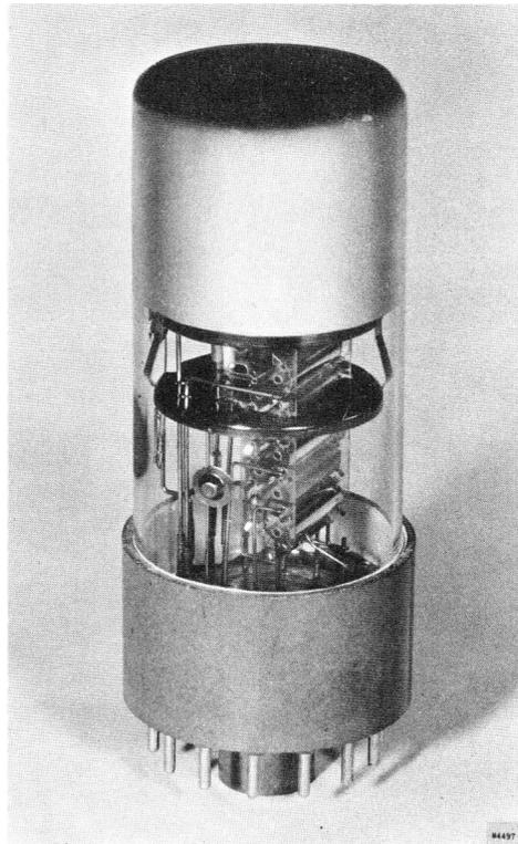
The 53 AVP is an 11-stage photomultiplier tube provided with a caesium-antimony semi-transparent flat cathode, which has a diameter of 44 mm.
